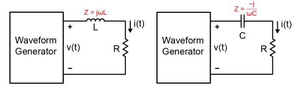
To these circuits we will apply sinusoidal, square, and triangular voltage waveforms. For all three you will measure both the voltage v(t) and the current i(t) and later find the power dissipated in the resistor. You can get the current through those elements by measuring the resistor voltage and dividing by the resistance. When the waveform generator is set to produce a sinusoidal voltage, you will also compute the power factor for the RL or RC combination.
