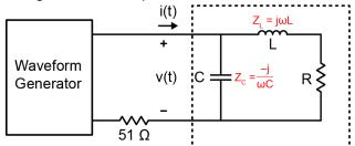
Measure the power factor for the R,L,C combination shown in the box. (As in Lab 2, you will need to measure two sinusoidal voltages, and apply Ohms law for the 51  $\Omega$  resistor to infer the current.) Adjust the frequency until the power factor is one. Record the determined frequency.
