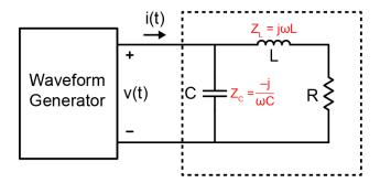
The total impedance of the R, L, C combination shown above is given by:
