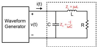
6. Simulate the circuit in the previous step using PSpice and plot the source current and the voltage across the resistor and the capacitor as a function of time. Again, choose a time range sufficient that the initial conditions do not matter. Compute the power dissipated in the circuit.
