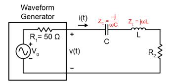
In order to completely describe this circuit, we must take into account that the waveform generator has an internal 50  $\Omega$  output resistance (denoted R1), which cannot be ignored. The phasor current is
