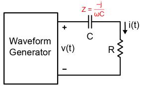
4. Use PSpice time-domain simulation to plot the voltage across R and C of the previous step as a function of time. For the PSpice simulations, use the "Transient Analysis", and choose your simulation time window to be long enough that your answer does not depend on the initial conditions.
